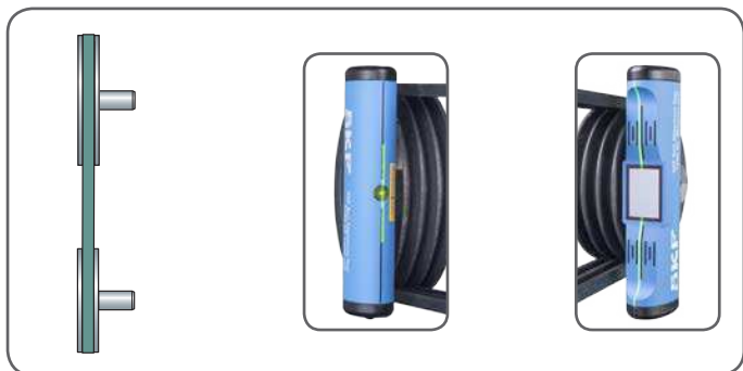
Figure 9 Pulleys perfectly aligned
